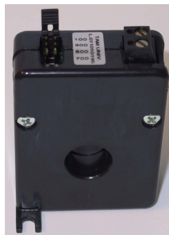
Fig. 1.1.1a. External TAM (current transformer) (required only for boards CP1* and CP3*)
