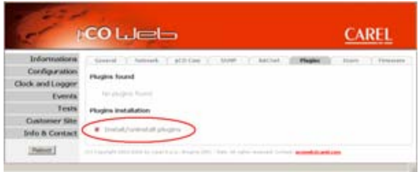
Figure 8.o – Plugin page: pCOWeb has found one or more Plugins to be installed
