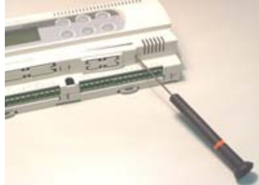
Figure 2.b – Removing the cover from the pCO controller
