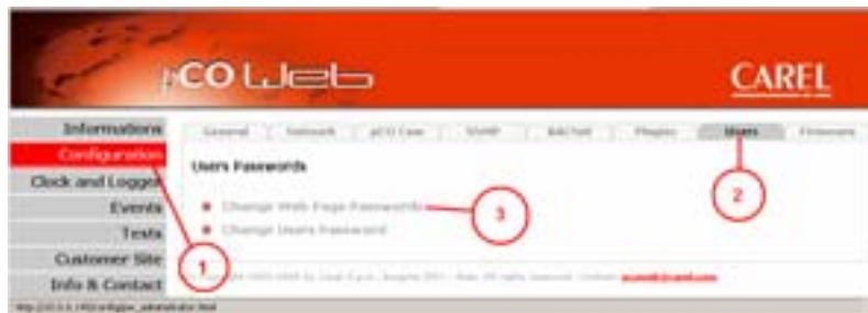
Figure 8.w – Protection and access control
