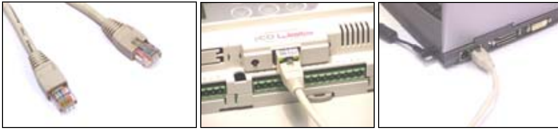
Figure 3.f – pCOWeb - PC connection
