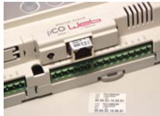
Figure 2.d – Securing pCOWeb with the cover
