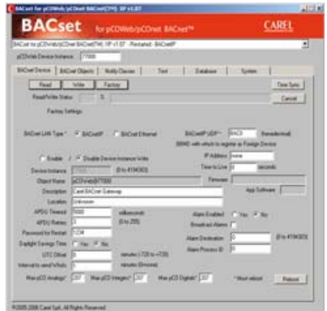
Figure 7.b - BACset software for the advanced pcOWeb BACnet configuration
