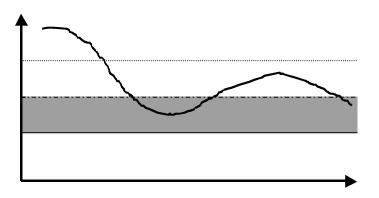
Function enabled with the value of the parameter OSH too high. The advantages of the function are not exploited adequately.
