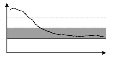
Function enabled with the optimum value of the parameter OSH. Except for sudden variations in the load or disturbance in the system, the showcase will remain in ON for a longer time than with traditional control, yet with a temperature and relative humidity that are much more stable and nearer to the set point. - *Def.*: 0.0.
