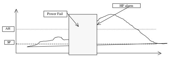
When an HA or HF alarm is activated, the display shows the codes "HA" or "HF", the alarm LED and the HACCP LED come on, the buzzer sounds and the alarm relay is activated.
