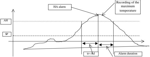
"**HF**" – this is activated after a power failure if, when power returns, the temperature is higher than the threshold of "AH" + "St". The following data are saved:
