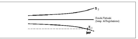
In this case, in fact, the temperature control is based on a "weighted" value of the two probes (S1 and S3). This means that despite the fact that the reference is constant, the temperature of the two probes may in reality differ significantly, with the risk of having an evaporator air outlet temperature (that is, the air that comes into contact with the product) that is dangerously low.
