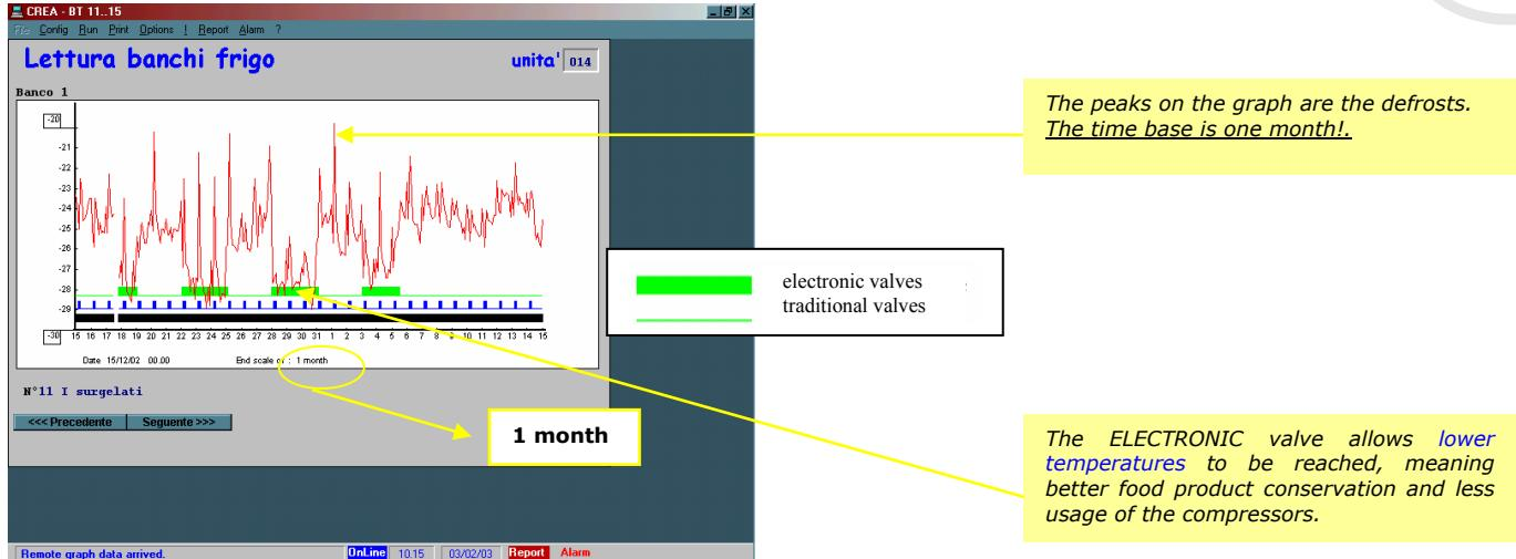
Fig. 12: Operating temperature of the utility: "frozen food island" in the PERIOD from 15 Dec-15 Jan
