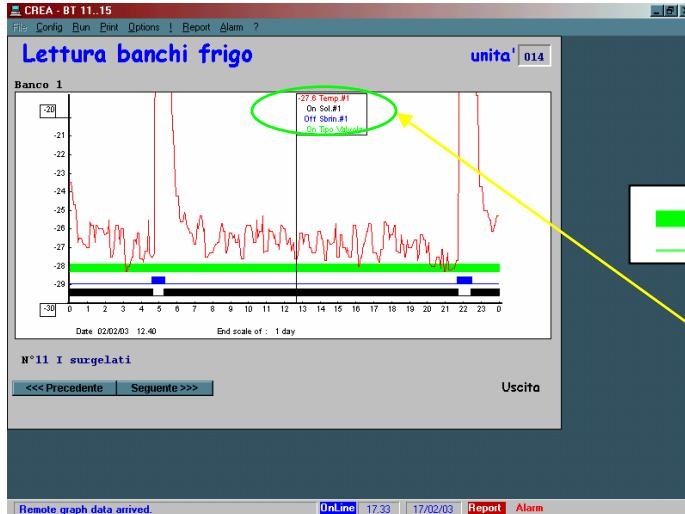
Fig. 14: Enlargement on a DAILY scale of the operating temperature of the frozen food island no. 11 operating with an ELECTRONIC VALVE.
