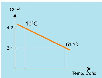
Fig.2: COP values with evap. temp. (-10°C)
