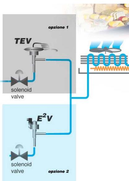
Each of the refrigeration utilities (showcases and coldrooms) has been installed with a **double parallel circuit** managed by a solenoid valve, which can at any time have the utility operate using one or the other technology. This allows a direct comparison of the two technologies (TEV and EEV) for the same operating conditions.
