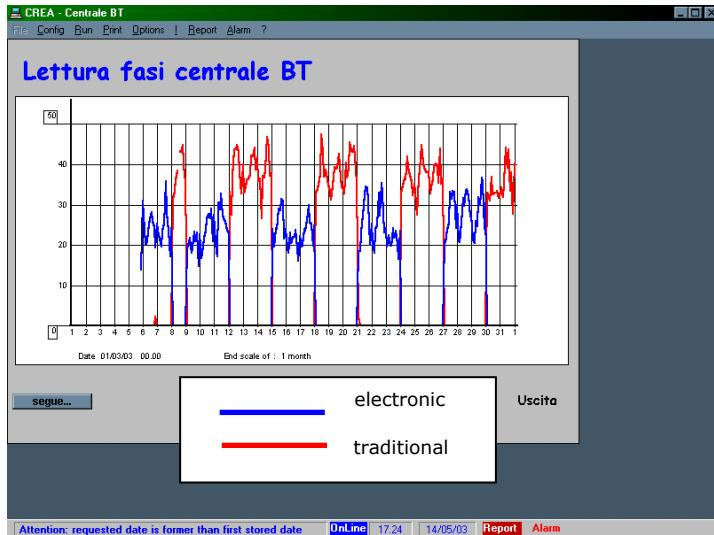
Fig. 10: Power consumption data corresponding to the month of MARCH 2003
