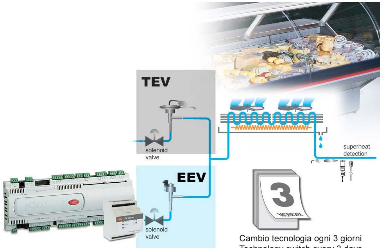
Fig. 6: dual technology (TEV-EEV) diagram for each refrigeration utility
