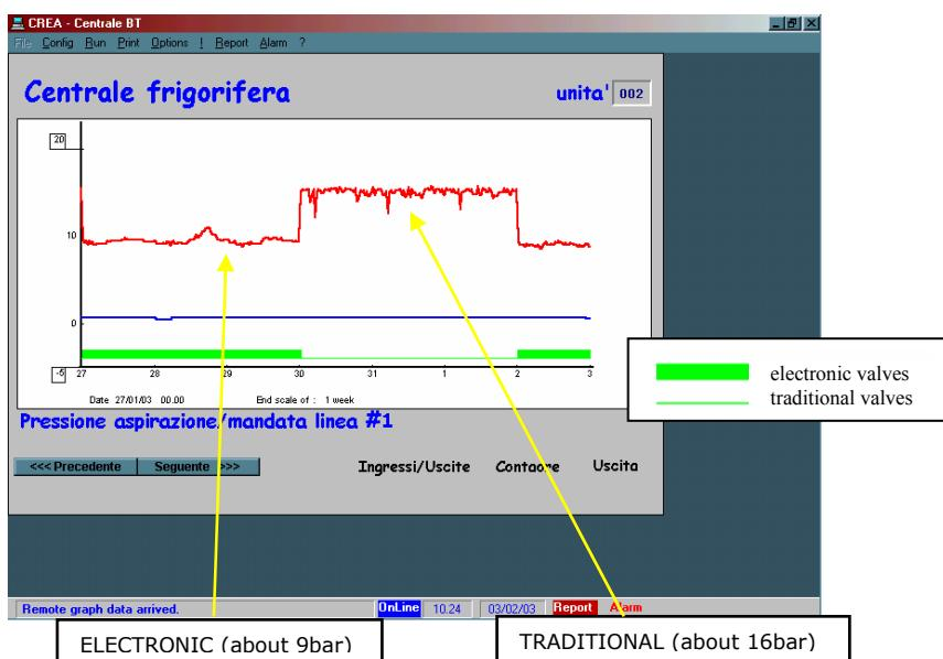
Fig. 11: Data on the compressor pressure in the LT refrigeration system corresponding to the WEEK from Jan 27 to Feb 3, 2003
