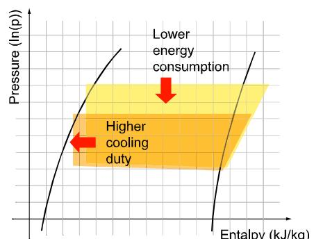
Fig. 3: pressure/enthalpydiagram
