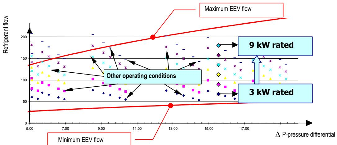
The graph shows the capacities of various compressors (from 3 to 9kW in rated conditions for air-conditioning<sup>5</sup>): the larger dots represent the rated conditions.
