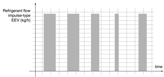
Another remarkable difference between proportional and PWM EEVs is the propagation of pressure pulsations on the refrigerant lines, particularly in case of long piping (ex. Supermarkets application) and in presence of heat liquid-gas heat exchangers. Pressure pulsation may lead to unpredictable faults not really in the EEV itself but in the general piping system (liquid line, evaporator, distributor, heat exchanger,...).
