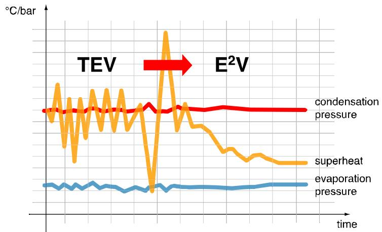
→ The lowering of the superheat set point often means an increase in the capacity delivered by the unit due to the consequent increase in the evaporator pressure and the better use of the exchange surface of the evaporator<sup>8</sup>.
