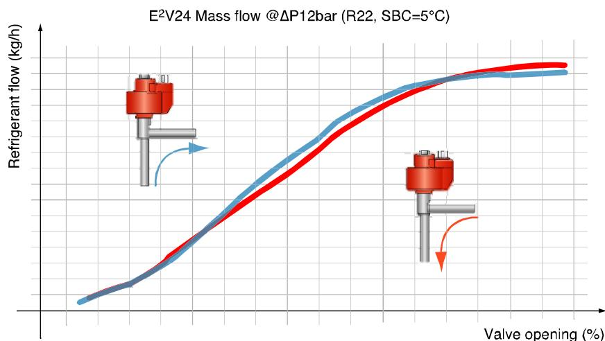
The almost perfect linearity of the flow is evident at both high and low degrees of opening.
