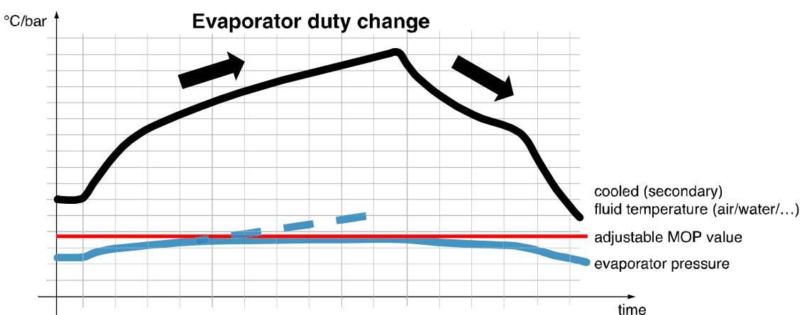
The typical action of this control routine is the progressive closing of the expansion valve, so as to limit the evaporator pressure: this intrinsically involves an increase in the superheat value and the temperature of the gas at the evaporator outlet (the temperature of the superheated gas or the suction temperature).
